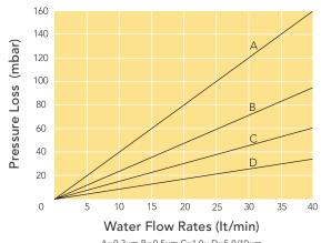
$A=0.3\mu m~B=0.5\mu m~C=1.0\mu~D=5.0/10\mu m$
