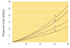
Air Flow Rates (m<sup>3</sup>/hr @ 0 barg) A=0.3μm B=0.5μm C=1.0μm D=5.0/10μm
