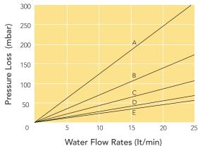
A=0.03μm B=0.1μm C=0.2μm D=0.45μm E=0.65/0.80/1.0µm
