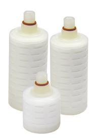
The use of a naturally hydrophobic membrane in **SupaPore TP** cartridges helps prevent the filter from wetting-out during use. This is critical in applications where water vapour is present to ensure that air flow into and out of the equipment is maintained. Typical applications include tanks containing liquids at elevated temperatures and autoclaves where steam may come into contact with the filter.
