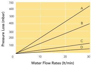
A=  $0.5/1~\mu m$  B= $5/10~\mu m$  C= $20/30~\mu m$  D= $50~\mu m+$
