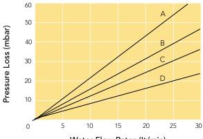
Water Flow Rates (It/min)  $A = 0.5/1 \ \mu m$   $B = 5/10 \ \mu m$   $C = 20/30 \ \mu m$   $D = 50 \ \mu m + 10/10 \ \mu m$
