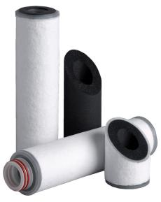
The SupaCarb CP carbon block uses a unique sintering process that combines both granular and powdered activated carbon. This results in the highest available surface area for adsorption of contaminants. The carbon block is protected by a spun-bonded, pure polypropylene fibre prefiltration layer, to produce a unique high performance module, offering superior on-stream life.
