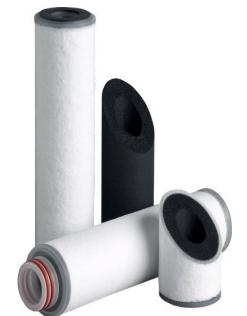
The construction of SupaCarb RP/XP uses a polyester substrate, unlike many other rolled elements that use a cellulose based support. This minimises the risk of microbiological contamination and because of its better compatibility it can be used in a wider range of chemical applications.
